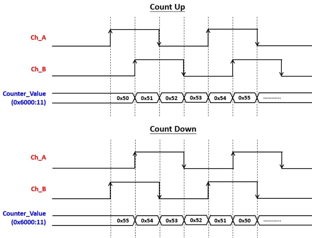
Figure 6.24 Encoder Mode – A/B Phase 4X)
