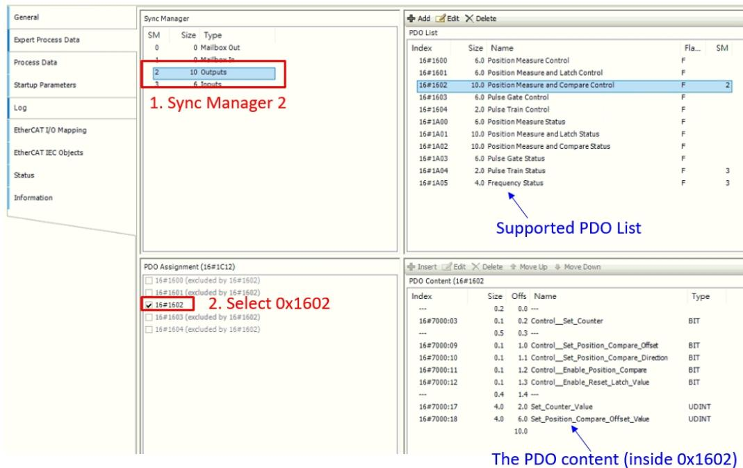
Figure 6.22 PDO assignment for SM2 - CODESYS interface
