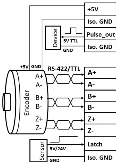
**Figure 6.17 Wiring for AMAX-5081**
