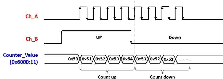
Figure 6.25 Encoder Mode – Pulse/Direction
