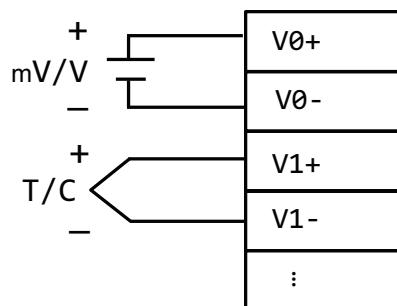
**Figure 4.25 Wiring for AMAX-5018**
