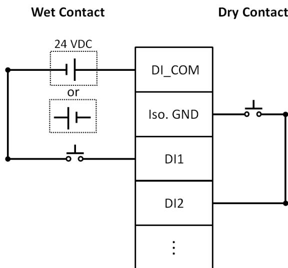
**Figure 5.10 Wiring for AMAX-5052**
