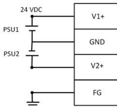
**Figure 3.7 Wiring for AMAX-5001 Power Input**
