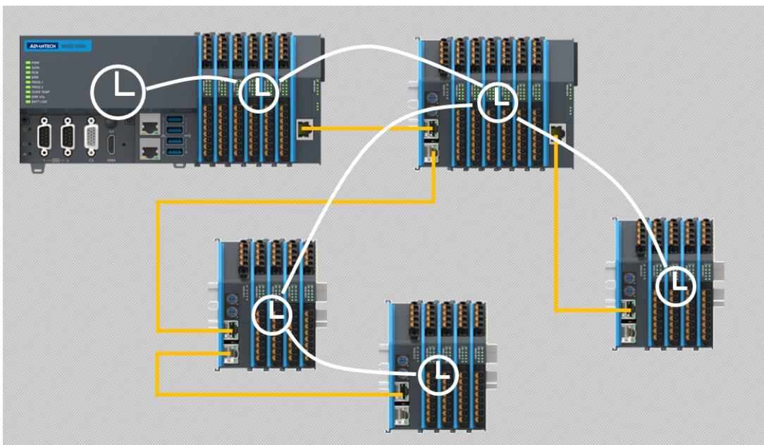
**Figure 7.3 EtherCAT Distributed Clock**
