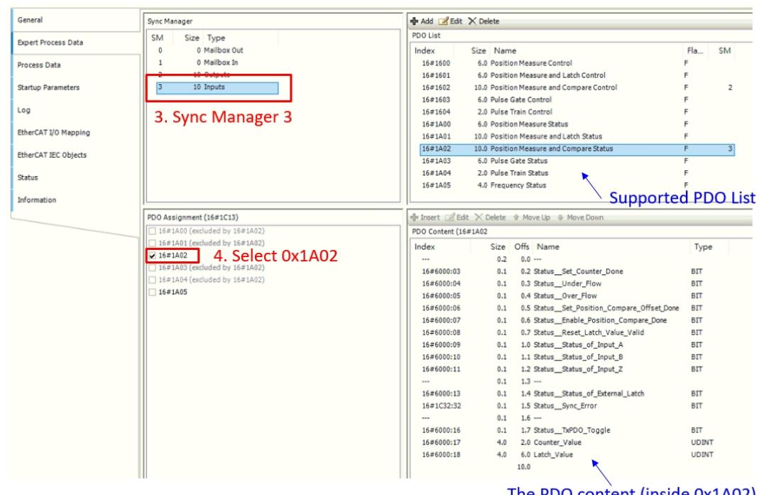
Figure 6.23 PDO assignment for SM3 – CODESYS interface
