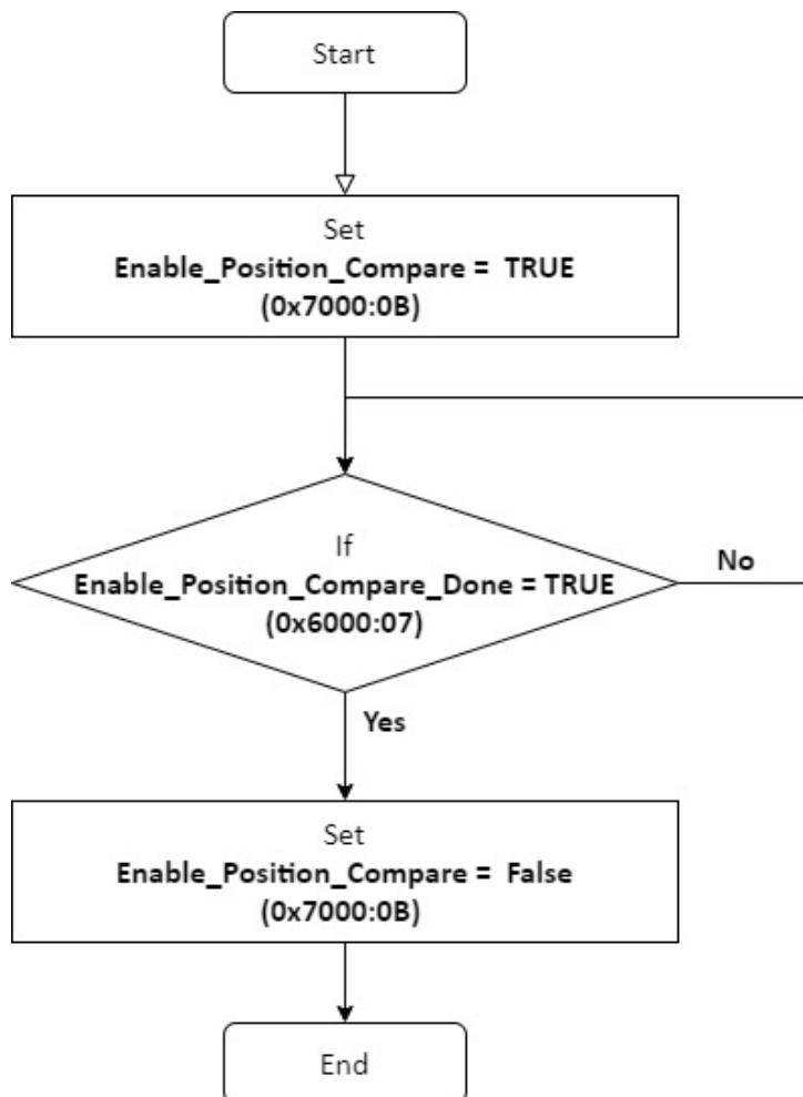
Figure 6.36 AMAX-5081 Hardware Position Compare Application – Flow Chart
