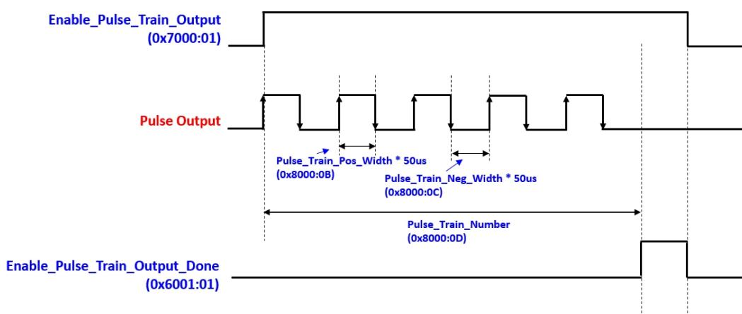
**Figure 6.28 Pulse Train Output**
