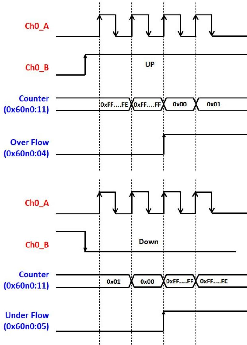
Figure 6.9 Counter Overflow and Underflow
