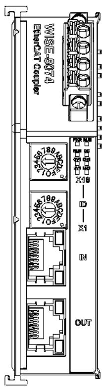
Figure 3.11 AMAX-5074 Module Front View
