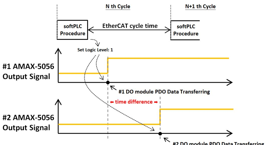
Figure 7.2 Standard Digital Output Module (SM mode)
