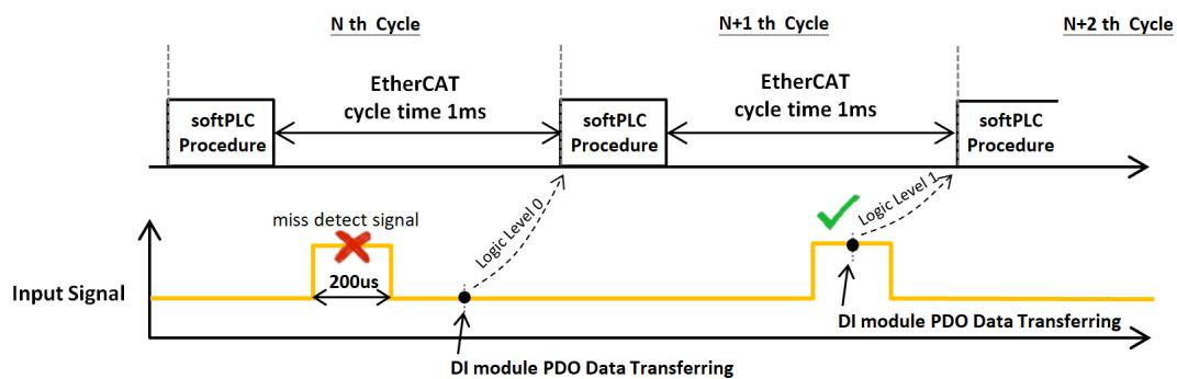
Figure 7.1 Standard Digital Input Module Signal Acquisition
