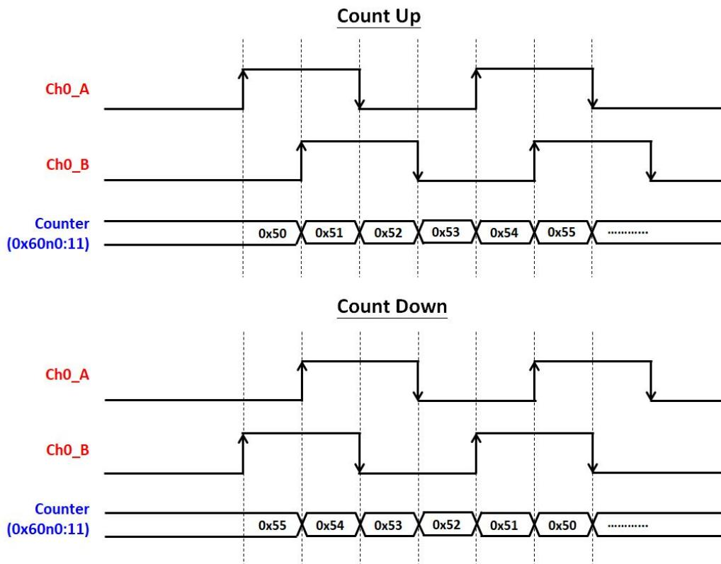
**Figure 6.7 Encoder Mode – A/B Phase 4X**
