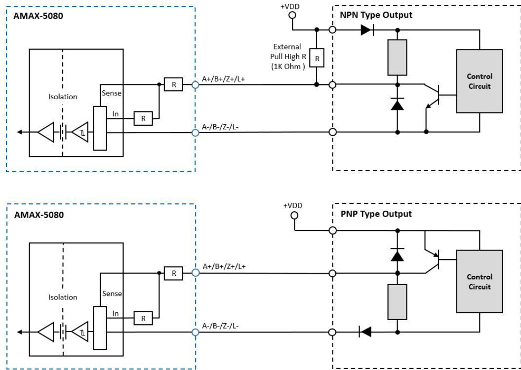
Figure 6.6 AMAX-5080 Encoder Input
