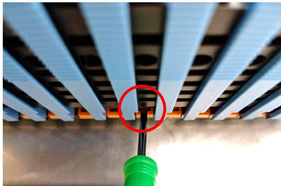
Figure 2.2 Unlock the latch to remove the module
