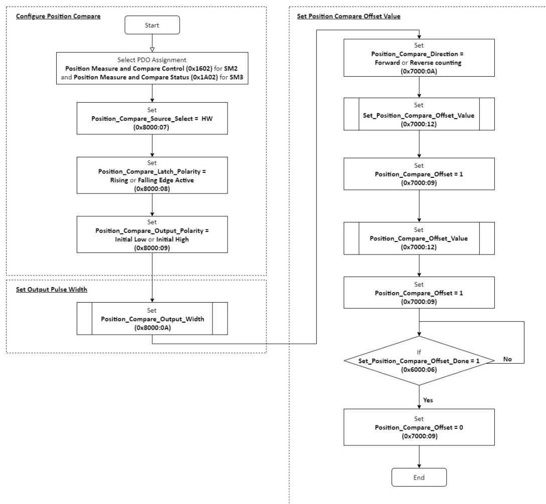
**Figure 6.34 AMAX-5081 Hardware Position Compare Configuration – Flow Chart**
