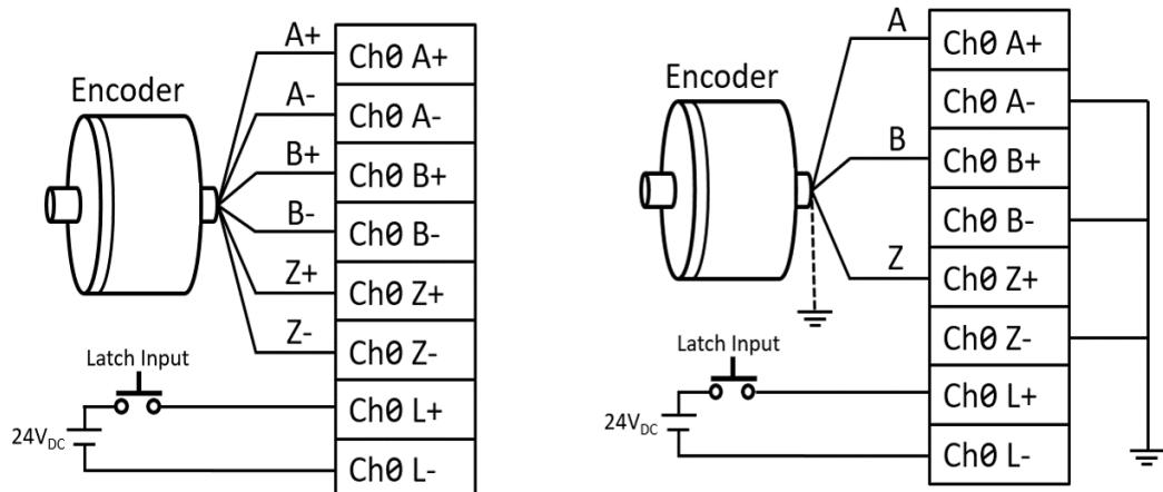
**Figure 6.5 Wiring for AMAX-5080**
