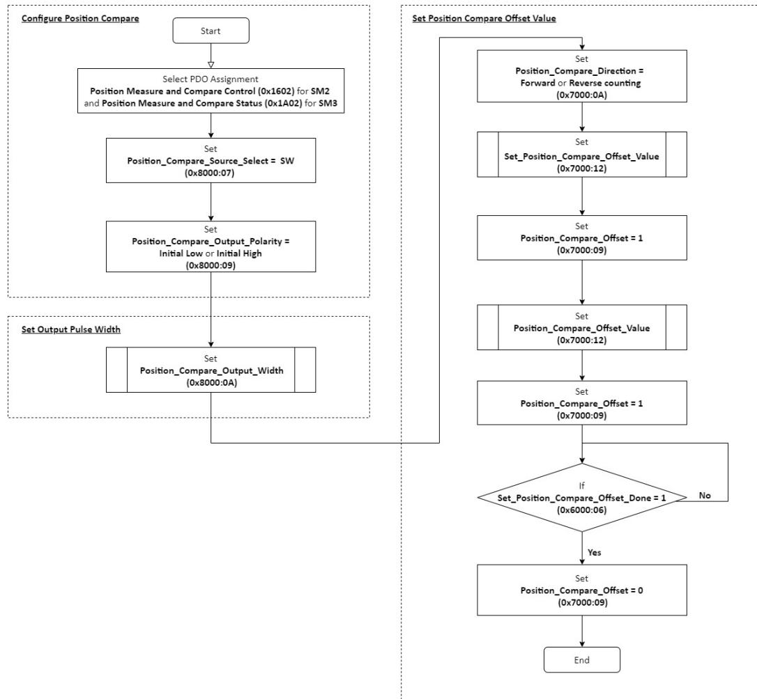
**Figure 6.38 AMAX-5081 Software Position Compare Configuration – Flow Chart**
