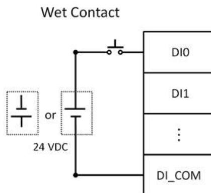
**Figure 3.6 Wiring for AMAX-5001 Digital Input**
