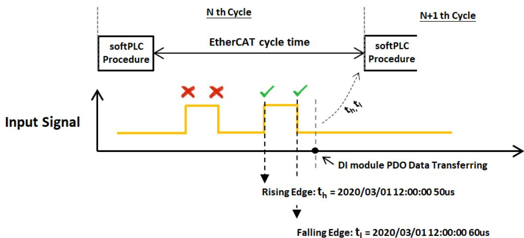
Figure 7.5 Digital Input with Timestamp - Continuous Mode
